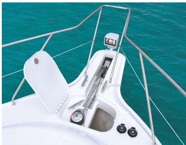
Handling ground tackle is a snap with the optional windlass, and the anchor well is roomy and deep.
